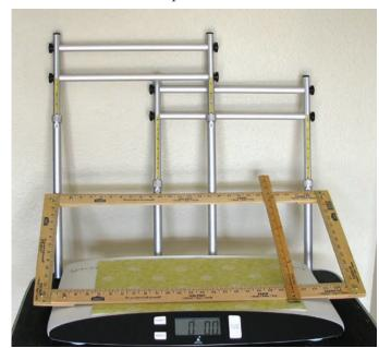
The measuring tools used were a Redmon Precision Scale, and two E-Z-wickets (10-17 and 17-31 inches) and Jon Coe produced a purpose-built device for measuring length using yardsticks.
